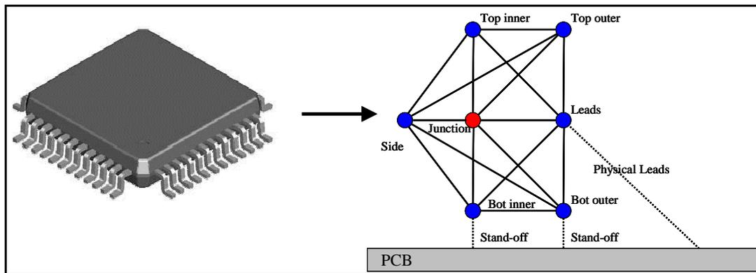
**Figure 4 — Possible node topology for a PQFP package**
